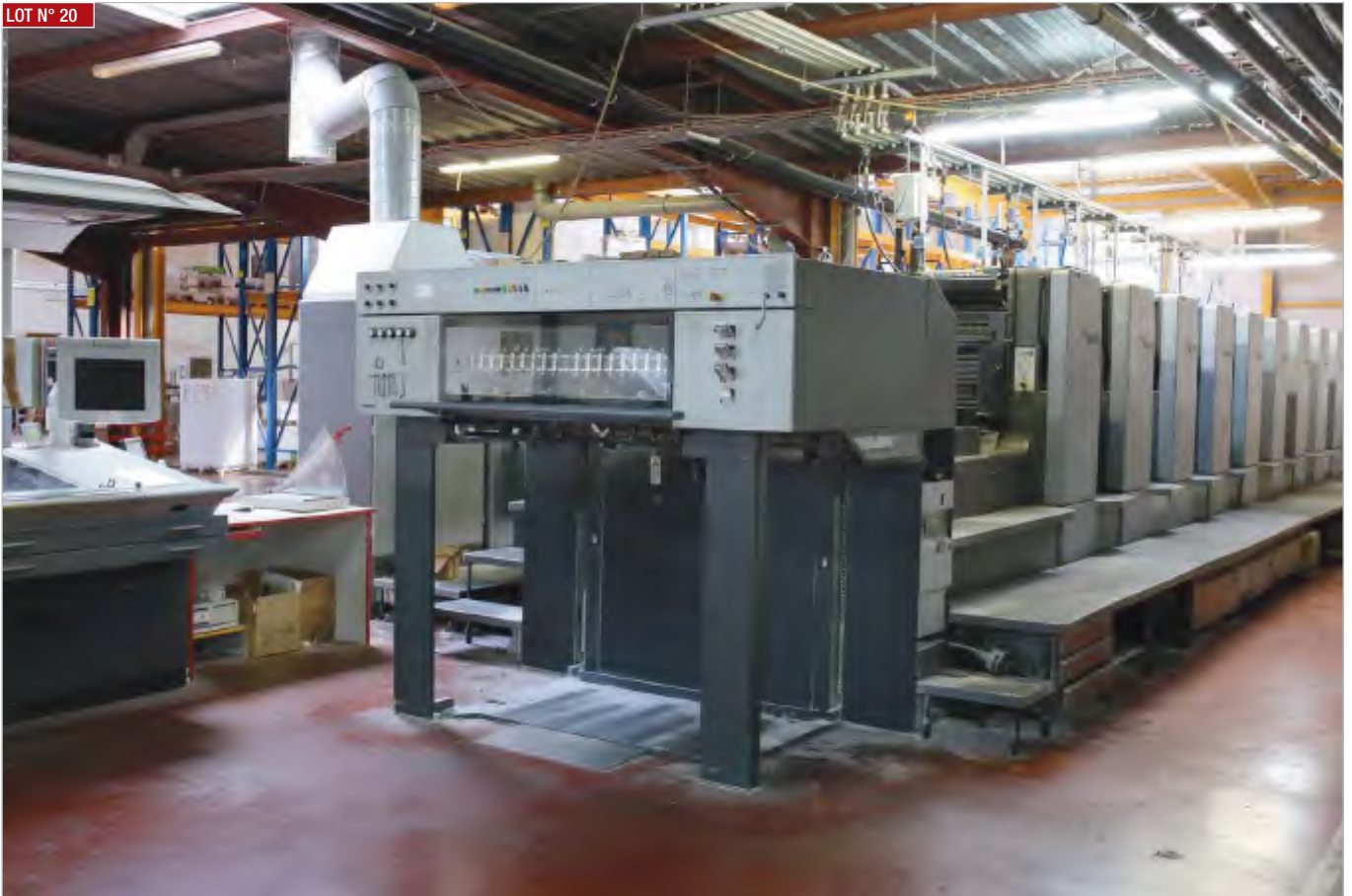
► Presse offset HEIDELBERG 10 couleurs, 72 X102 cm, mod. SPEEDMASTER, type SM102-10-P6-S (2004)
